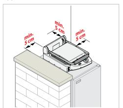
Position the appliance respecting the indicated distances in the diagram and so that the back of the oven is easily accessible for appliance connections and maintenance.
